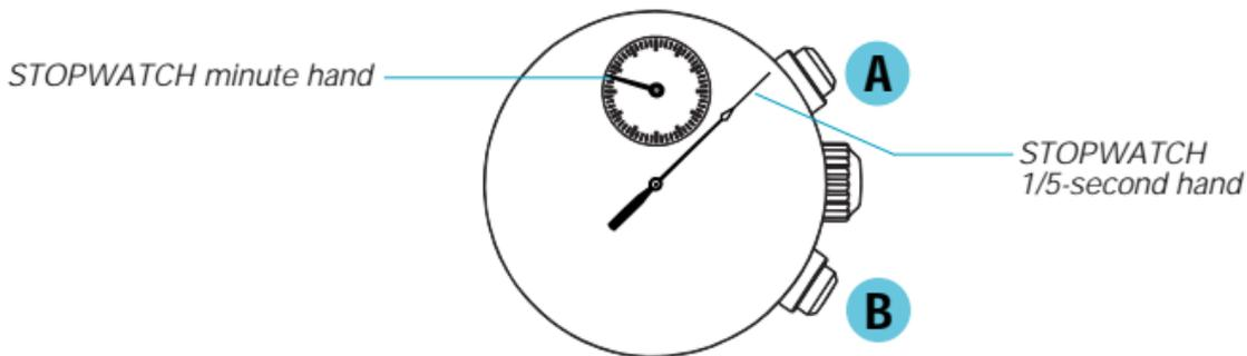
☆ Before using the stopwatch, be sure to check that the crown is set at the normal position and that the STOPWATCH hands are reset to the "0" position.
