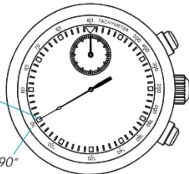
"90" (tachymeter scale figure) x 1 (km or mile)
