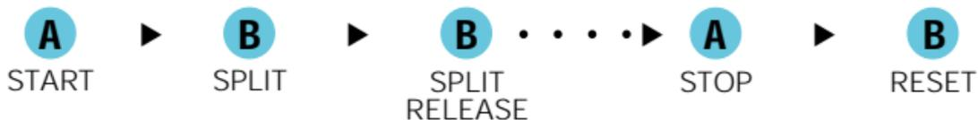
*\* Measurement and release of split time can be repeated by pressing button B.*
