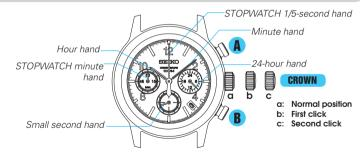
\* Some models may have a screw lock type crown. If your watch has a screw lock type crown, refer to "SCREW LOCK TYPE CROWN".
